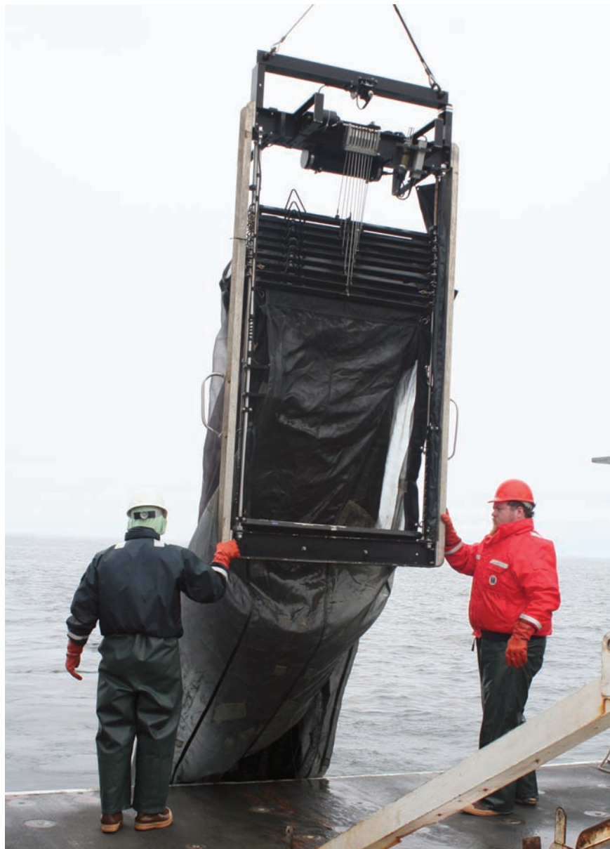
University of Alaska (UA)–Juneau graduate students Wesley Strasburger and undergrad Elizabeth Siddon operate the MOCNESS (multiple opening/closing net and environmental sampling system), a net that captures larger-sized zooplankton than does the CalVET net. After dragging the device, with its nine tapering nets, behind the ship, they spray it down and collect the fish larvae, krill, and other pelagic zooplankton to be identified. Photograph: © Wendee Holtcamp.
