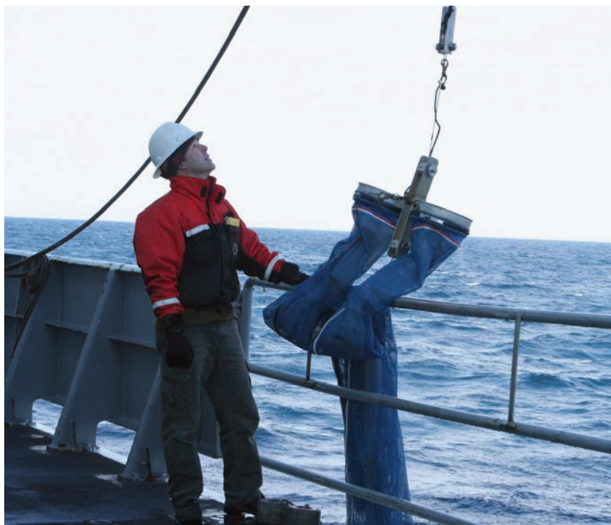
University of Alaska-Fairbanks Seward Marine Center oceanographer Alexei Pinchuk deploys a CalVET net, which resembles a giant pair of pants, over the starboard side of the ship, lowering it to just above the seafloor with a winch. He hauls it back up, sprays down the paired nets, and washes the “zoop soup” inside into containers. Photograph: © Wendee Holtcamp.
